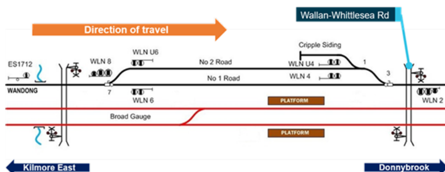
The rail track layout. Standard Gauge tracks are shown in black, adjacent Broad Gauge tracks are shown in red. Source: ARTC/ATSB
