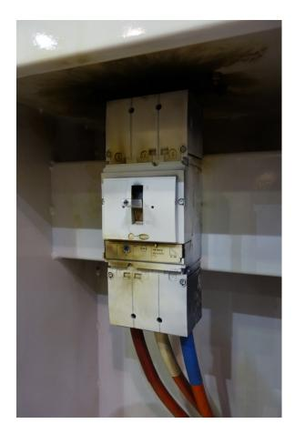
**Test 3** - Internal arcing-fault test at a prospective current of 50 kA rms at 415 V initiated on the load side of the MCCB (standard test). Fuse wire was 20A. There were minimal effects inside the compartment and no effects on the door. There was a small flash visible before interruption of the fault by the MCCB.
