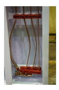
**Test 2** - conditional short-circuit current of 50 kA rms at 415 V on a 3 pole MCCB (moulded case circuit-breaker). The Circuit breaker limited the trough fault current and magnetic forces on the cables connected on the load side. The blackening on the breaker was due to the material ejected from the arc chutes of the breaker.
