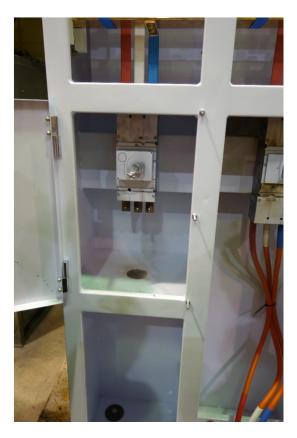
**Test 4** - Internal arcing-fault test at a prospective current of 50 kA rms at 415 V for 0.2 s initiated on the line side of the MCCB (special test). Fuse wire was 20A. Part of the busbars on the line side of the MCCB disintegrated. The MCCB handle was propelled off the door, and some of the door fixings and hinges were damaged or broken.
