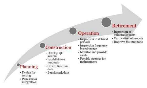
Fig, 5 Role of NDT in various stages of life cycle management of an asset
