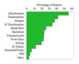
Figure 4. Solar cell degradation reported statistics.
