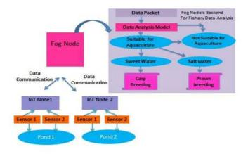
Figure 3: Fog Computing Based fishery Application
