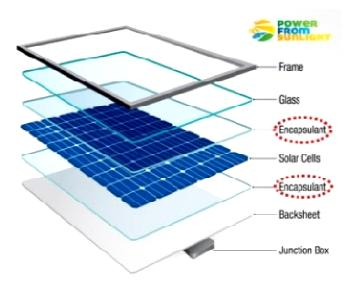
Figure 1. Components of the solar panel [4].
