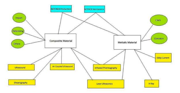
Fig 1 The boxes in yellow signify the NDT techniques. The ovals in green signify the type of defects that could appear
