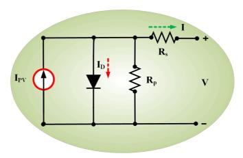
Figure 1. Single diode solar cell model
