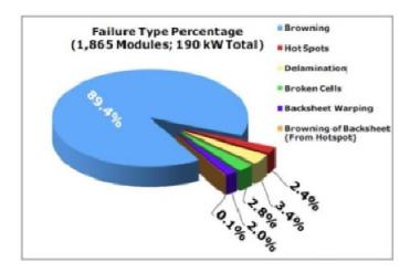
Figure 3. American solar cell degradation modes [7], [8].
