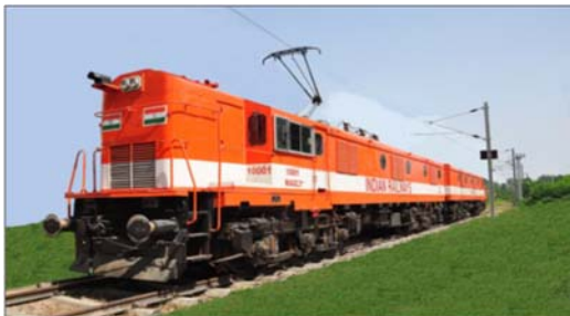
Converted twin Co-Co Electric Loco WAGC3
