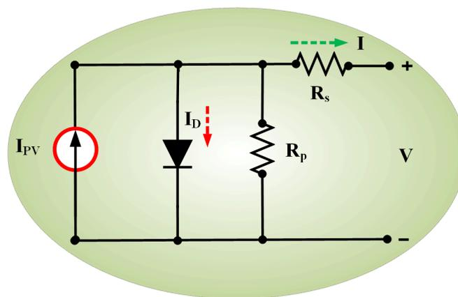
Figure 1. Single diode solar cell model
