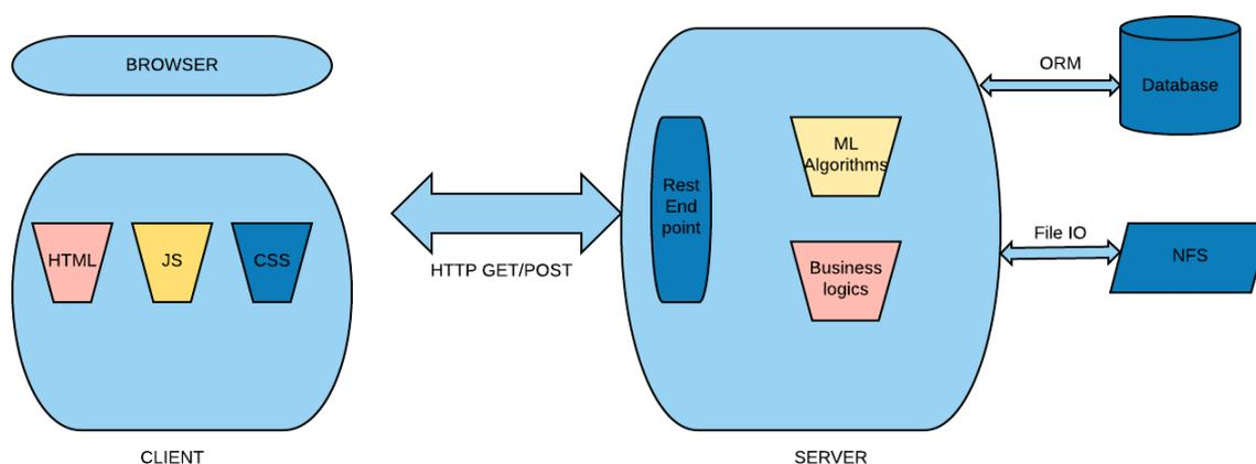
As shown in the Diagram above, Django is based on MVC architecture. Below are the main components:
