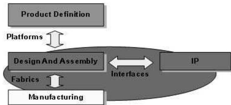
Figure1. Electronic System Design
